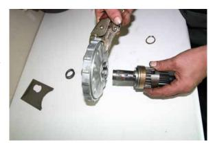
Carefully remove all gears and the o-ring from the main shaft.
