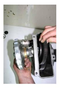
Holding the brake assembly using the mole grips, remove the circlip from the end of the shaft. Remove the brake from the shaft and place in a safe place.
