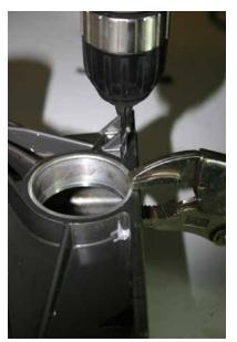
Once the shim is positioned, secure using a suitable clamping device (e.g. mole grips)
