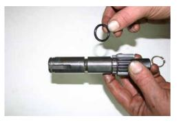
Remove drum from lower housing and clean all parts thoroughly. The original main shaft can now be discarded.
