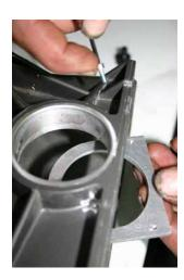
Refit drum and large gear to lower casing, and locate modified retention plate inside casing.
