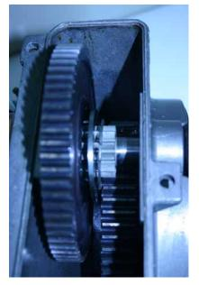
Now insert the main shaft, taking care to fit the large intermediate gear, round shim and circlip. (flat side of the round shim faces circlip)
