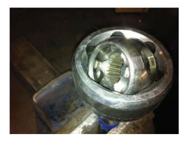
Rotate the cage inside the cv socket so it is standing vertical, line the 2 opposite openings in the cage up with the cv socket walls and the cage will lift free from the housing. This may take some persuasion.
