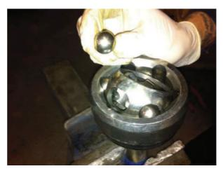
Move around the cv working in opposites until all the ball bearings are removed.
