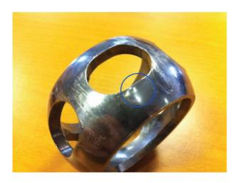
Use a die grinder with a metal cutting tool to remove the high spots and to restore the components to there original shape, test fit the components together and check for ease of movement. the components should move smoothly and not bind tight.
