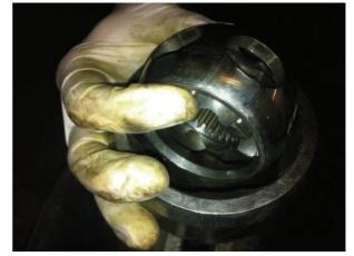
Once the cage is free from the cv socket rotate the inner spider until the outer land of the spider lines up with the openings in the cage, the spider can now be rolled out the bottom of the cage keeping one of the lands located in one of the cage openings.
