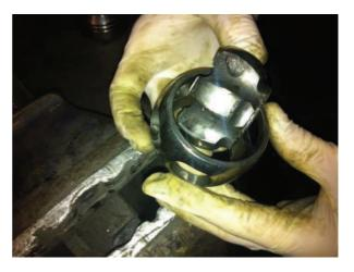
(The bottom of the cage is the end with the larger inner opening and closest to the openings where the ball bearings locate, the top of the spider inner is recognised by the flats on the ends of the lands.)
