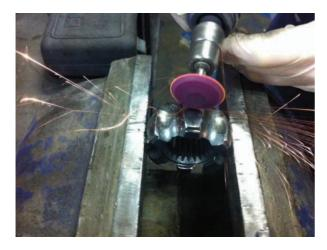
Change the metal grinding tool in the die grinder to a flapper type tool and finish the previous ground areas to a smooth finish, refit all components in reverse order to removal and check for smoothness.
