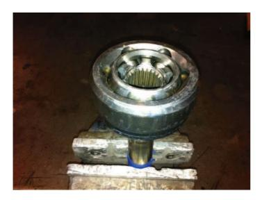
To remove to ball bearings use a soft punch (aluminium) and a hammer and strike down on the outer cage directly above a singular ball bearing location. With some persuasion the ball bearing opposite to this location will rise to its highest point and come free from the cage, remove the ball bearing and repeat the striking process on the opposite ball bearing location.
