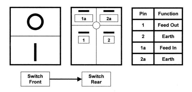
Only one earth connection is required on the switch. Use either terminal 2 or 4 for the earth.
